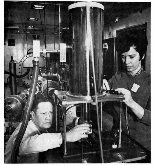
PHYSICIST RUTH WHAN (5211) attaches thermocouple wires to monitor sample temperatures during irradiation on the Van de Graaff accelerator while R. S. Neiman hooks up an electrical connection to monitor radiation levels.
